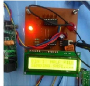
Figure 3: Result 2 showing Garbage level is Half filled
