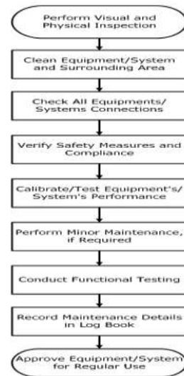
Figure 7.3.1: Preventive Maintenance Flowchart
