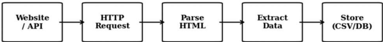
Fig. 4 — The web scraping pipeline: from website to stored dataset
