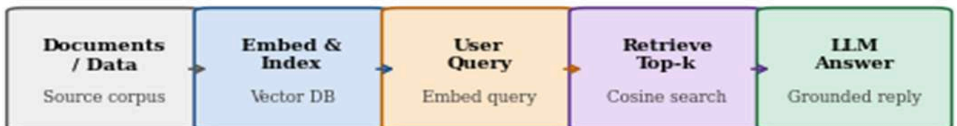
Fig. 4b — RAG pipeline: documents are embedded and indexed; at query time the top-k chunks are retrieved and sent to the LLM
